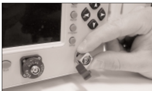
Figure 10. Removing the EUI
