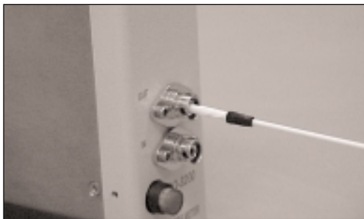
Figure 6. Cleaning bulkhead connectors
