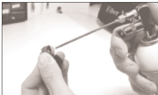
Figure 12. Drying the EUI with compressed air
